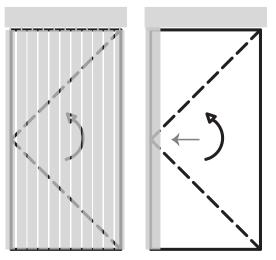
For vertical blinds on a casement inswing to operate the window you slide the blinds over to the far side opposite the handle. We put a 4" limit on all windows so the blinds will not be in the way of the sash operating.
