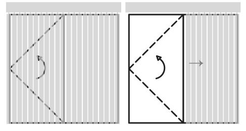
For vertical blinds on a casement inswing beside a fixed window, to operate the sash the blinds would simply slide over to the fixed side.
