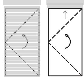
For horizontal blinds on a casement inswing the blinds would be installed above the top of the window. To operate the window you pull the blinds up.
