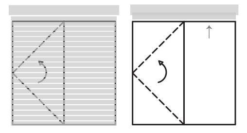
For horizontal blinds on a casement inswing beside a fixed window the blinds would be installed above the top of the window. To operate the window you pull the blinds up.
