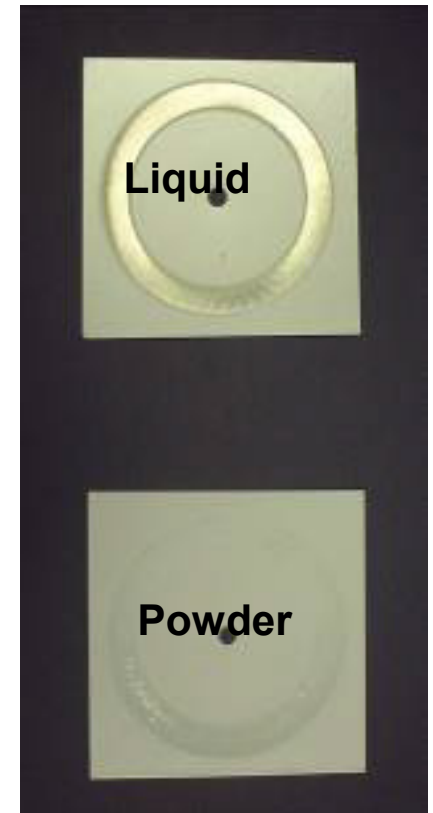
Comparison of abrasion test results show liquid visibly has more wear.
